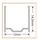
Name Straight aluminum channel Code LN1010-SC Material Aluminum Mounting style Surface mounted Length 1m Width 12.4mm Height 13mm Internal width /
