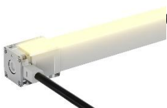
ARVO-L-MEC-LS-2P Mechanical end cap with screws, left side entry with 30cm (0.98ft) cable, 2 pin
